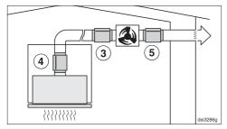
To minimise noise from the motor in the kitchen, the silencer should be positioned in front of the external motor (3) if possible, or, if the ducting is long, above the exhaust connection inside the rangehood (4). In the case of an external motor located inside the house, fitting a silencer behind the external motor (5) reduces the noise of the motor outside the house.
