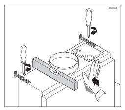
Align the housing and screw on the retaining brackets.
