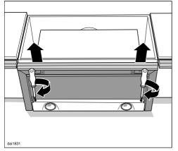
Use a screwdriver to align the deflector plate correctly.
