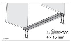
Secure the spacer strip underneath the housing unit sides, flush with the rear wall.
