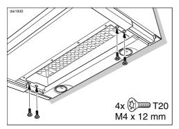
Secure the rangehood to the brackets from below using two screws on each side.
