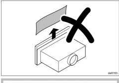
To avoid scratching the deflector plate, do not remove the protective film between the deflector plate and the casing until the rangehood has been placed in the housing unit.
