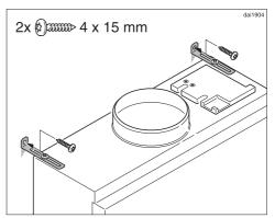
Secure the retaining brackets to the rear wall using the screws supplied.
