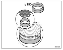
Secure the exhaust ducting to the exhaust connection, e.g. with a hose clip (available as an optional accessory) on flexible ducting.
