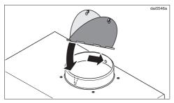
If required, install the non-return flap. Check that the flap opens easily and closes by itself. Depending on the model of rangehood, the non-return flap may already be installed.
