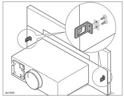
When fitting a 90 cm wide rangehood in a 60 cm wide wall unit, whilst the deflector plate is pulled out, unscrew the two deflector plate spring mounts.
